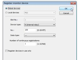
2. R100 is registered and is displayed on Device Monitor screen.
